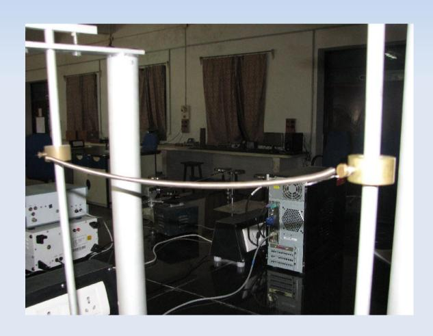
• Displace both the pendulums SLIGHTLY in one direction by the same amount to excite the in-phase normal mode. Calculate  $T_1$  and  $\omega_1$  for 20 oscillations.
